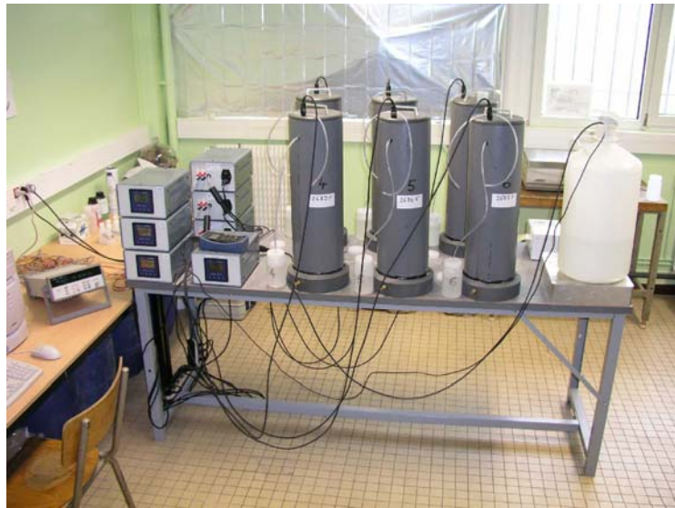
Figure 1. Experimental device with the six leaching columns
